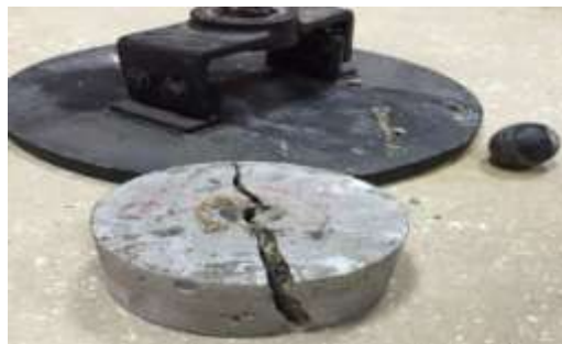
Fig. 7. Rubberized Concrete Impact Failure.
