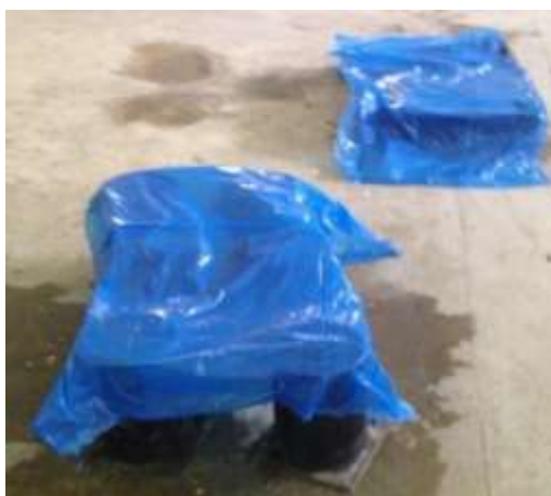
Fig. 3. Cylinders Covered in Plastic Sheets for Curing.
