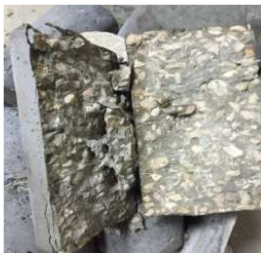
Fig. 14. Non-Rubberized Concrete Cylinders Splitting into Two Halves.
