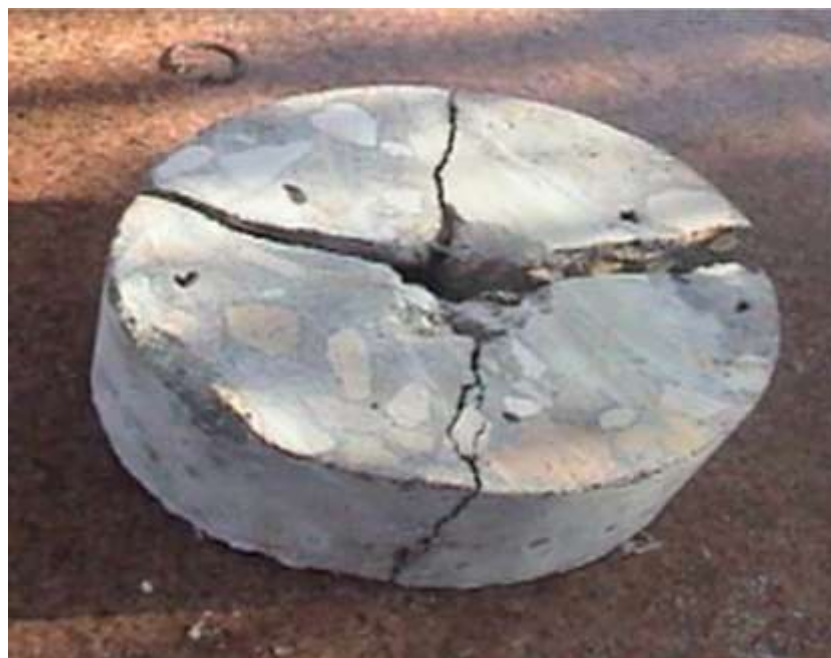
Fig. 8. Plain Concrete Impact Failure.
