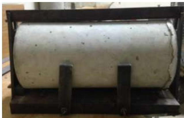
Fig. 4. Cylinder Placed in the Steel Strips.
