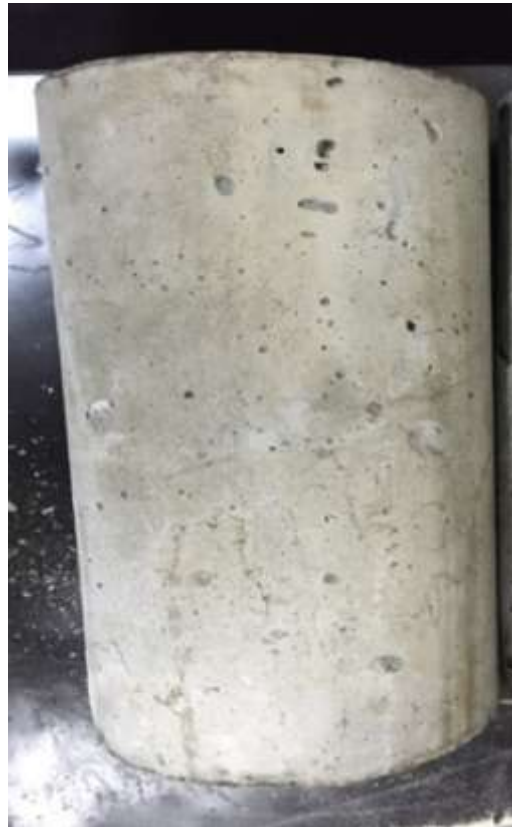
Fig. 15. Rubberized Concrete Cylinders without Splitting After Failure.
