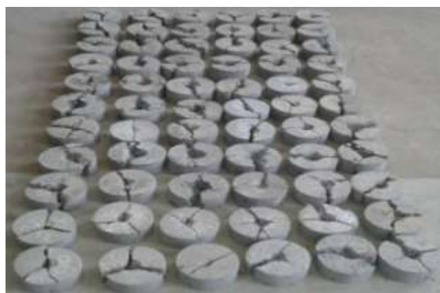
Fig. 9. Portion of the Specimens Subsequently to Impact Load Failure.
